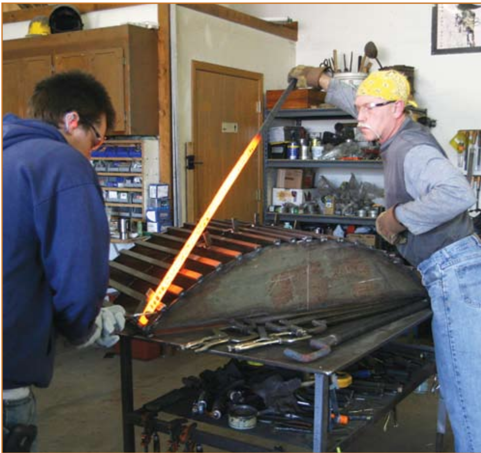
Benson and helper bend a railing frame piece on a form built specifically for this staircase.
