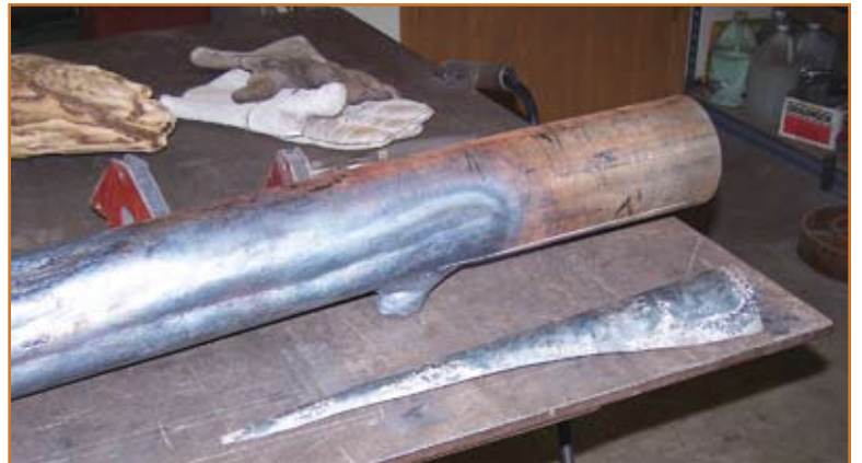
Newel post in process. Benson welded sheet metal pieces on to a pipe base to flare the bottom of the tree stump.
